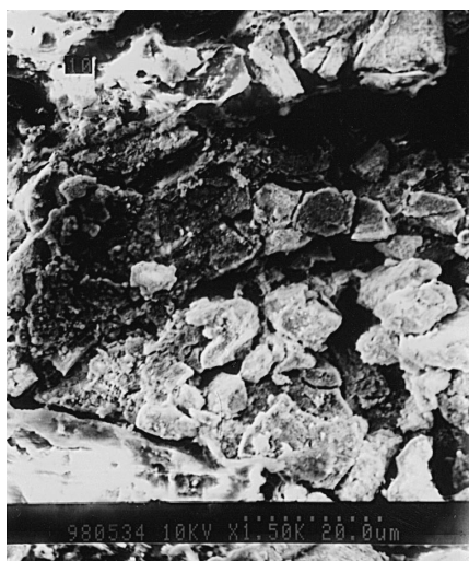
Fig. 4. Electron micrograph of electroless nickel-plated alloy particles in a MH electrode after 500 cycles.
